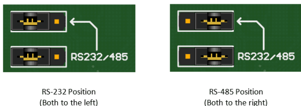
Figure 13 - detail depiction of RS-232 / RS-485 jumper positions
