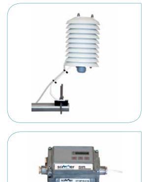
clear and cloudless nights, the surface temperature of the snow can sink below the air temperature so altering the snow crystals. The SIR sensor makes it possible to recognize and measure such situations which provides usefull information especially for avalanche forecasts.
