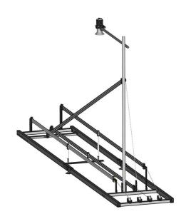
Determination of snowpack-properties can be very challenging as they vary significantly in space and time. The SPA-2 snow pack analyzer measures the volumetric contents of ice and water within a snowpack, and together with the snow depth calculates the snow water equivalent (SWE) and snow density.
