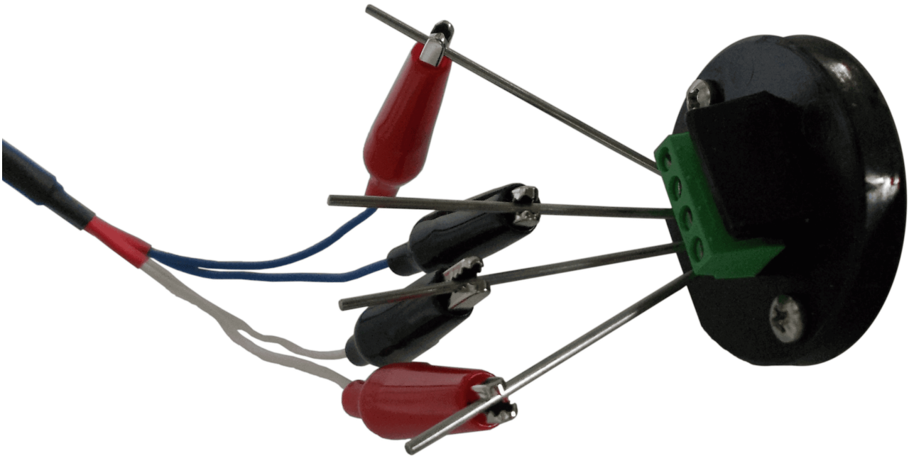
Figure 3 - Reed switch connections
