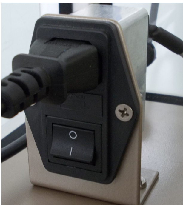
Figure 2 - Power switch in cabinet of TBRG Calibrator
