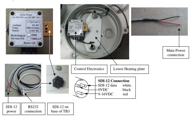
If SDI-12 communications is required, then connect the logger or RTU to the 3 pin connector (Switchcraft brand) on the base of the TB3 raingauge, and supply SDI-12 power.
