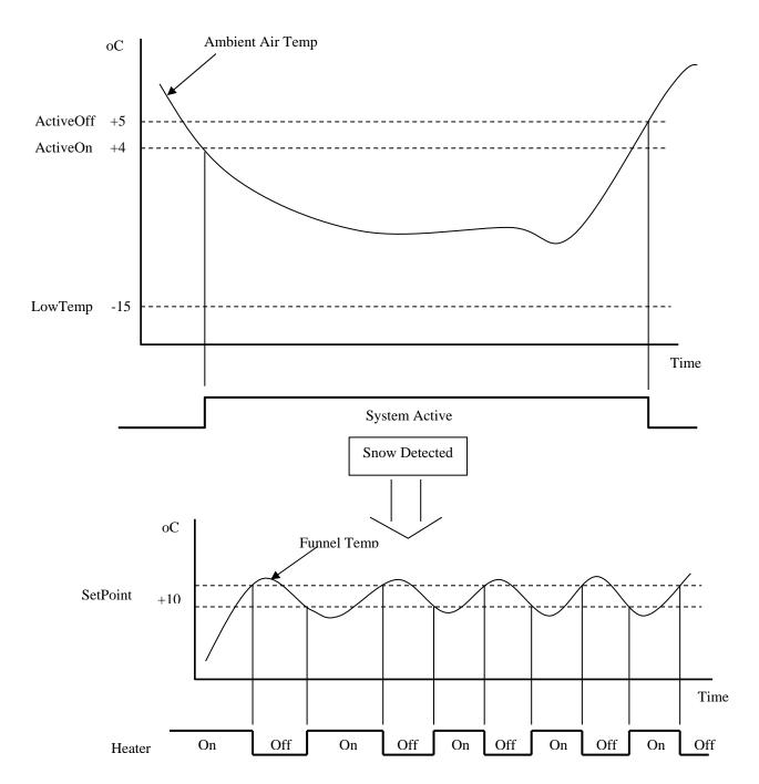
Diagram showing how the "Snow Run-On" timer controls the heater.
