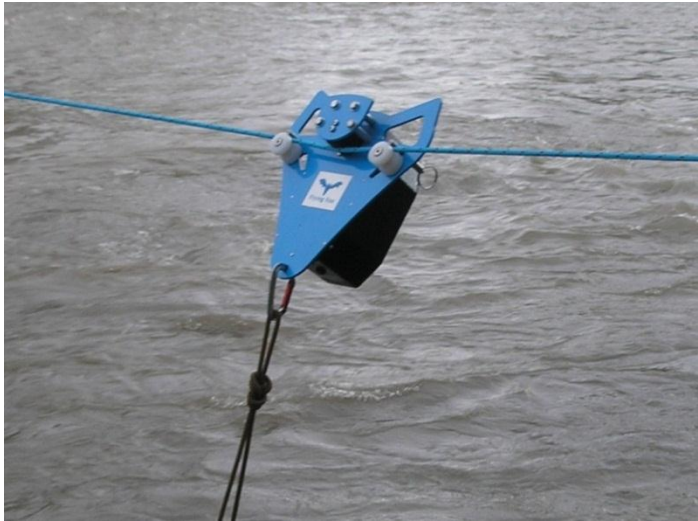
Figure 6. The Flying Fox installed on an optimally-tensioned span rope
