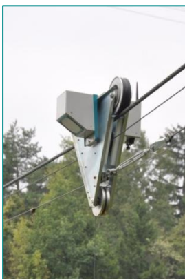
Figure 24: RP-30 mounting on a cable way
