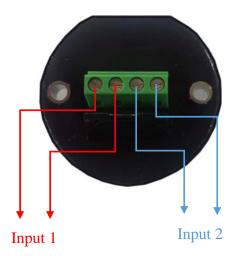
Note: 2x Digital inputs with maximum capacity of 24 Volts (0.5amp max.). They operate simultaneously to two different RTU's (example Data logger & Satellite modem)
