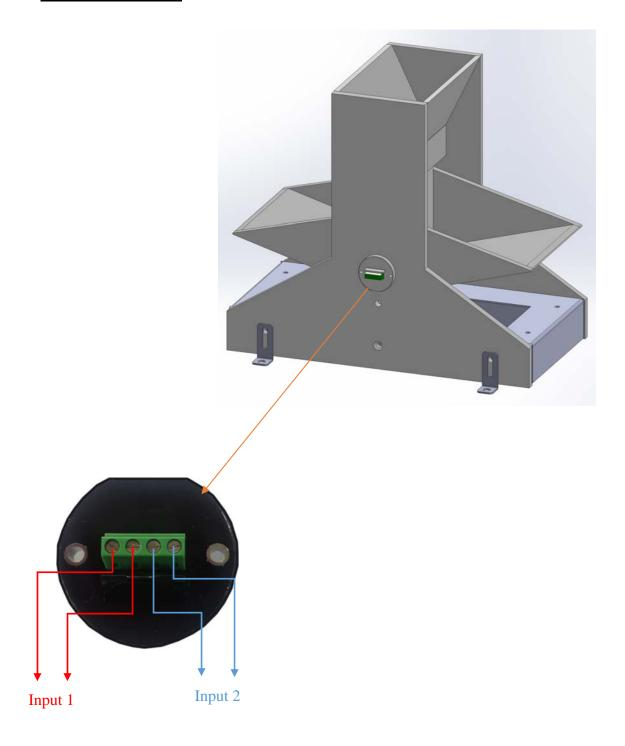
Each signal from this reed switch indicates a 0.5L or 1L of water flow depending on bucket size.
