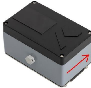
Figure 8 – HyQuant lid with indication of the reed-switch position
